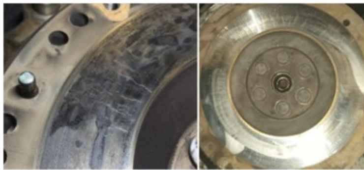
Examples of wear and overheating marks.
