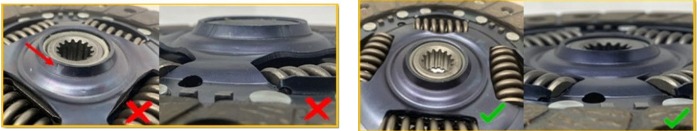
Left: conical deformation and cracks caused by forcing assembly. Right: a new disc in good condition.
